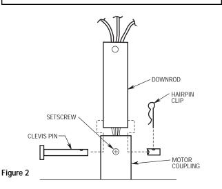
**3.** While pulling up on the downrod, securely tighten the setscrew in the motor coupling (Figure 3).
